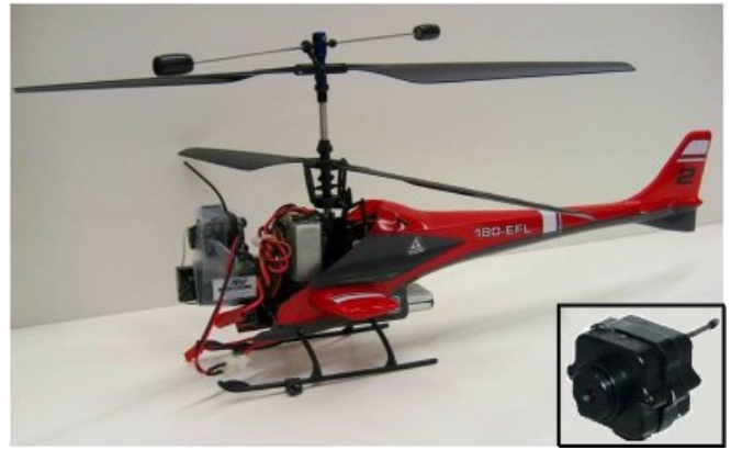
Fig. 3. Our co-axial indoor platform (inset shows the camera used).
